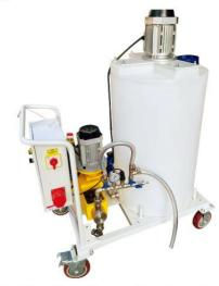
**Quick-Setting Pump Design for Gypsum Based Fireproof coating**
